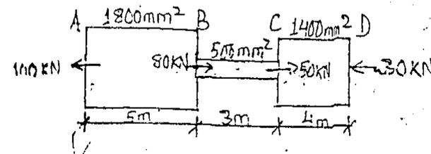
Determine the tensile and compressive forces in the different sections and also the total elongation of the bar. [Take  $E = 80 \text{ GPa}$ ]
